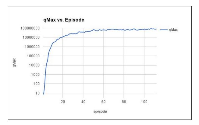
Here, qMax is the mean over all steps in an episode of the maximum Q(s,a) values generated for the state in that step. The graph shows that after about 30 episodes the action-value function converges.
