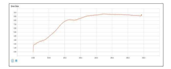
The above graph shows the mean Q-max value vs number of episodes trained for. Here, Q-max is the mean over all steps in an episode, of the maximum Q-values for a given state and all possible actions.
